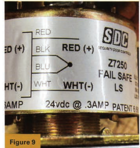
Figures 8 and 9. Here's the wiring diagram that can be found on the body of the lock for both 12 VDC and 24 VDC.
