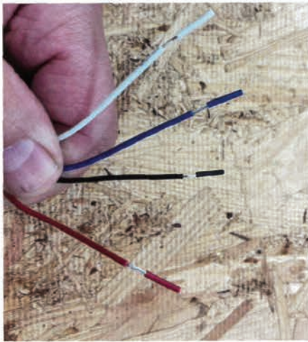
Figure 11. The PR-7200 regulator has four wires: white, blue, black and red.
