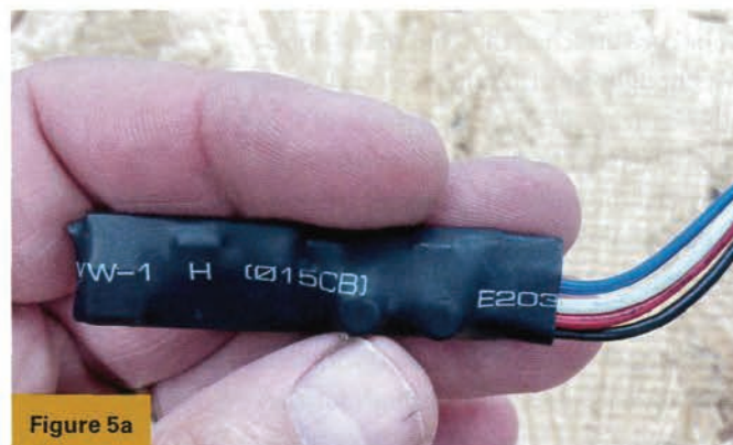
Figures 4-5a. The author chose the SDC Z7250GQ Electra Pro because the power regulator (Figure 5a) is included with the lock.
