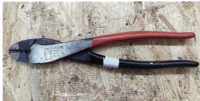
Figure 26. The author likes using these Sta-Kon (Thomas & Betts) crimping pliers.
