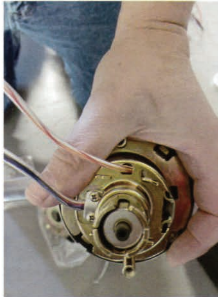
Figure 6. There are two cables coming out of the chassis of the lock body.
