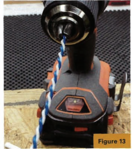
Figures 12 and 13. The author uses a drill to wind the wires together.
