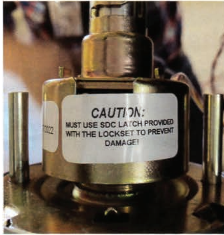
Figure 21. The manufacturer’s label indicates that the latch provided with the lock must be used.
