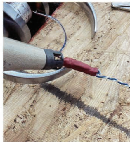
Figure 18. The author applied heat to the heat shrink tubing.
