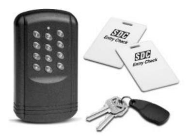
The EntryCheck® incorporates all the logic necessary to control a single door. All Unit Programming is performed by using the built-in keypad. Proximity cards, key fobs and PIN entries can be added and deleted with the keypad using the master code or programming card. The lock relay and auxiliary relay outputs can be set for 1-99 seconds.
