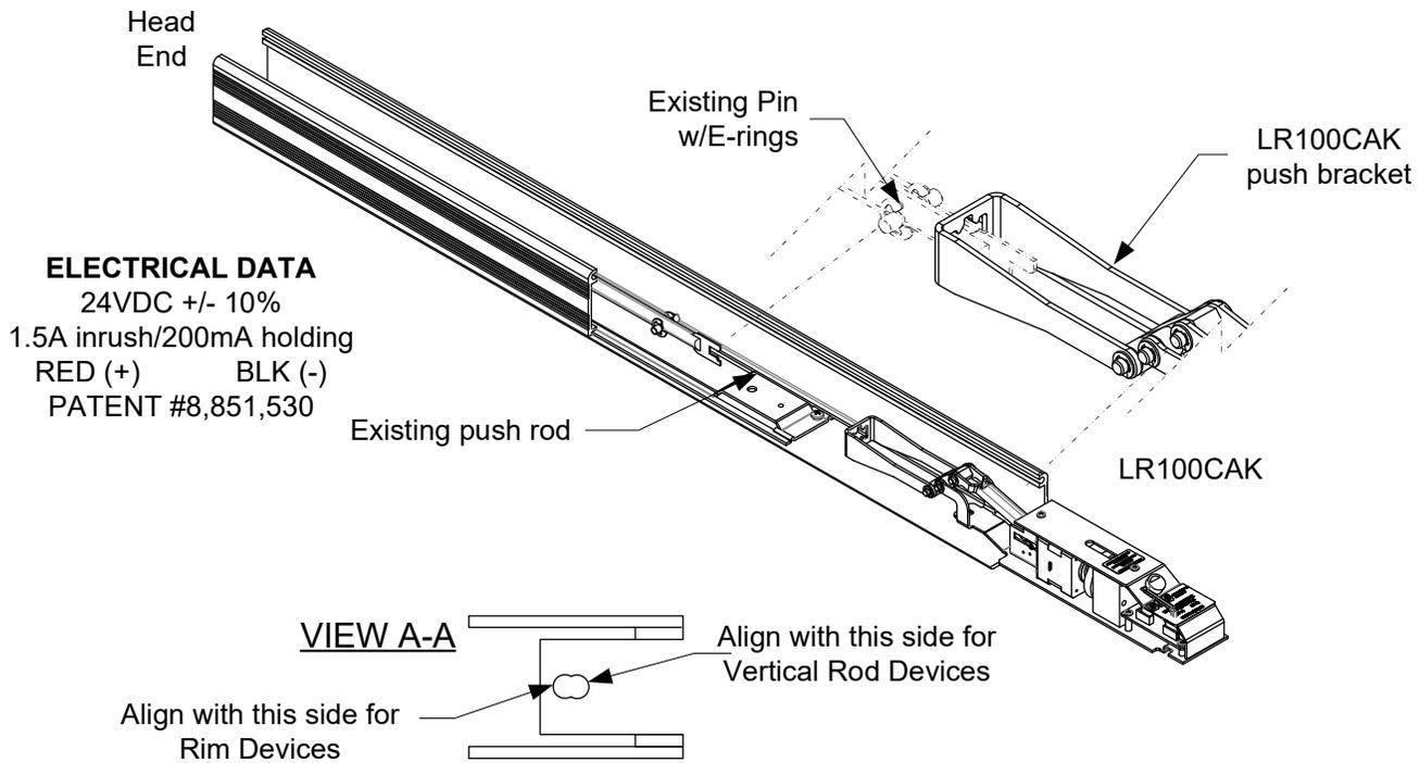
Align the desired mounting hole on the LR100CAK with the tapped hole on the push bar base plate and attach with the supplied screw/star washer. Test function and replace device cover and end cap.
