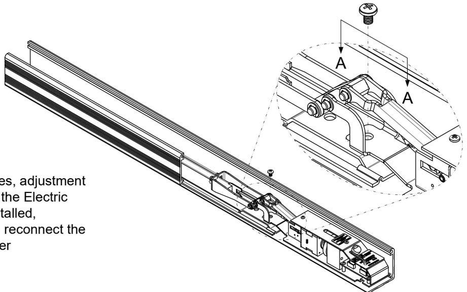
When retrofitting to existing vertical rod devices, adjustment of the rods is required for proper operation of the Electric Latch Retractor. Once the unit is properly installed, energize it so the latch is dogged down, then reconnect the vertical rods to the device and make the proper adjustments to the rods.
