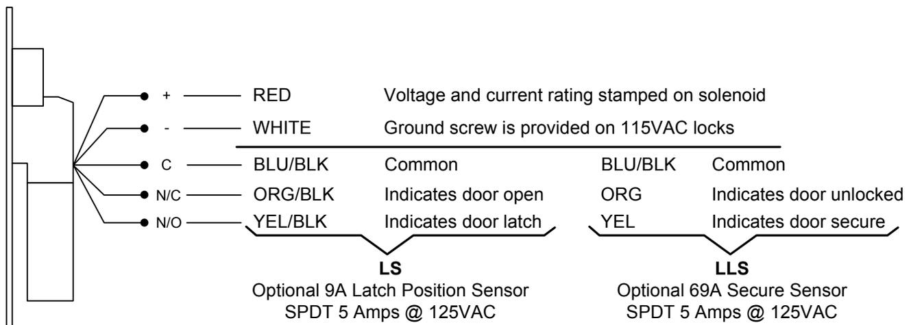
\* Wiring assignments for the optional SC-10 cable with socket connectors are the same
