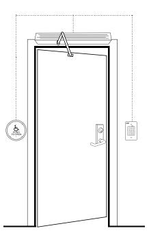
Mortise lock powered by operator MLR mortise lock retracts latch, allowing for door automation
