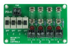
Power control modules ensure compatibility of access hardware components and simplify system installation and troubleshooting. Modules may be ordered with or without power supplies. Different modules may be specified for one power supply.
