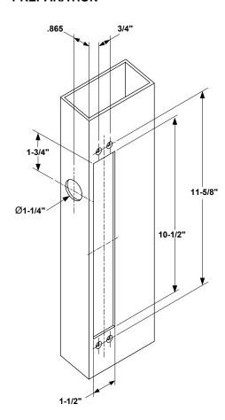
(8X) TAP TABS FOR #10-32 1-1/8" CYLINDER (NOT INCLUDED) Use standard straight cam ILCO (863G) or equivalent. Once the Key Cylinder is installed. Secure the cylinder within the Cylinder Locking quided cylinder slot Set Screw using the Cylinder Locking Set screw.
