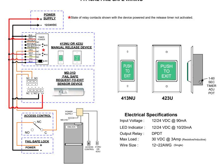
To be used with a Class 2 power supply or voltage compatible UL 294 or UL 603 listed power supply
