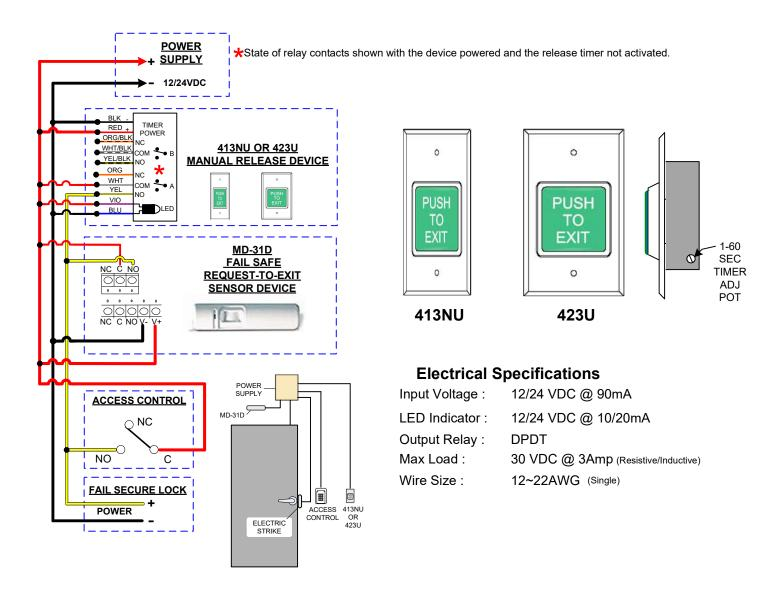
To be used with a Class 2 power supply or voltage compatible UL 294 or UL 603 listed power supply
