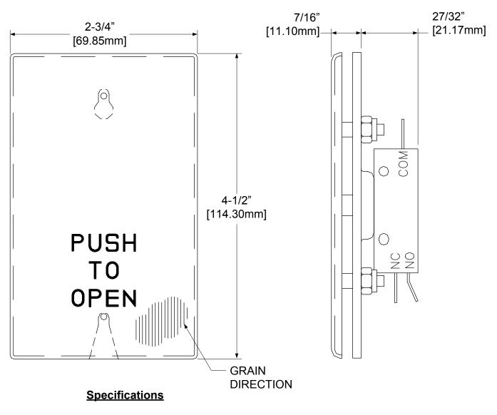
Physical Size: 4-1/2" x 2-3/4" x 1-9/32"D Switch mounts to a Single Gang or 2" x 4" electrical box
