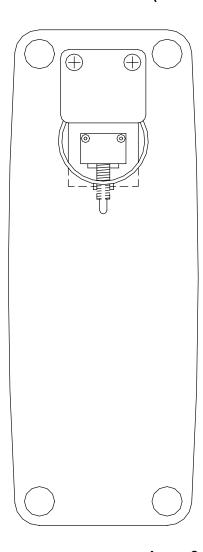
REMOVE TWO TOP ASSEMBLY SCREWS PLACE SWITCH ASSEMBLY AS SHOWN AND FASTEN SCREWS.
