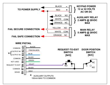
Fig. 4 Basic Door Installation Wiring
