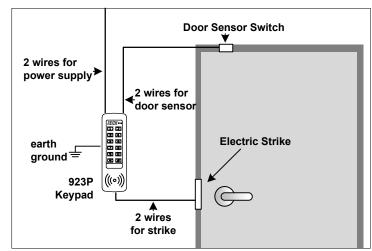
Fig. 3 Basic Door Installation
