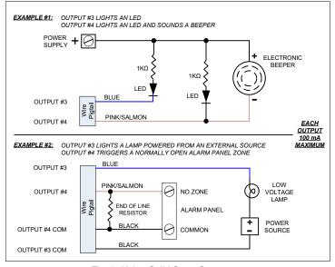
Fig. 5 Using Solid State Outputs
