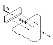
Install the new mounting plate using the existing mounting plate holes and the supplied hardware.
