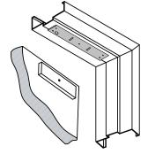
Locate the wire hole on the new mounting plate & drill a 3/8" dia. hole through the header.
