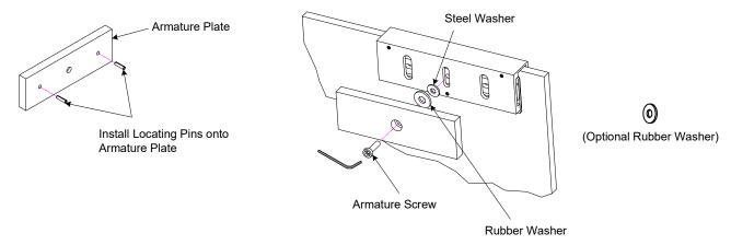
Adjust the Armature Adjustment Bar if required for proper alignment with the Armature plate and Magnet Lock surface. Once adjusted to the proper alignment, then fully fasten and secure the Armature Screw to the Adjustment Bar.
