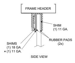
\* Second 11 GA. Shim Not Required For 5/8" thick Door Installs.
