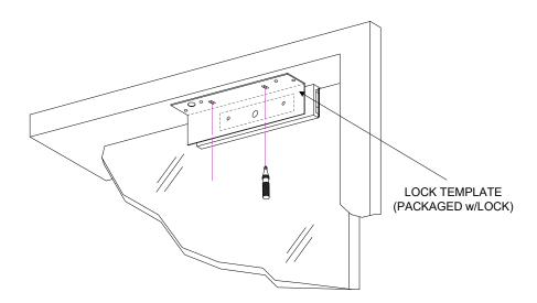
Install the Armature Plate to the Armature Adjustment Bar. The Armature plate and Locating Pins are supplied with lock (spare pins are also supplied with HDB1V kit). Use the Armature Screw that is supplied with the HDB1V kit to secure the Armature Plate. Do not fully tighten the Armature Screw.
