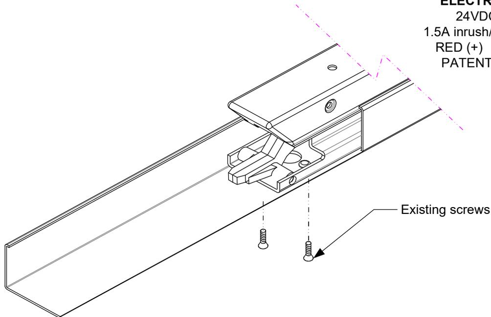
Slide the ELR assembly into the housing and under the hinge bracket. Position the roller at the front of the ELR under the pivot arm of the push bar.
