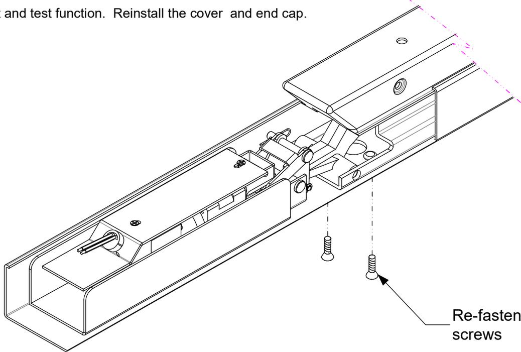
When retrofitting to existing vertical rod devices, adjustment of the rods is required for proper operation of the Electric Latch Retractor. Once the unit is properly installed, energize it so the latch is dogged down, then reconnect the vertical rods to the device and make the proper adjustments to the rods.
