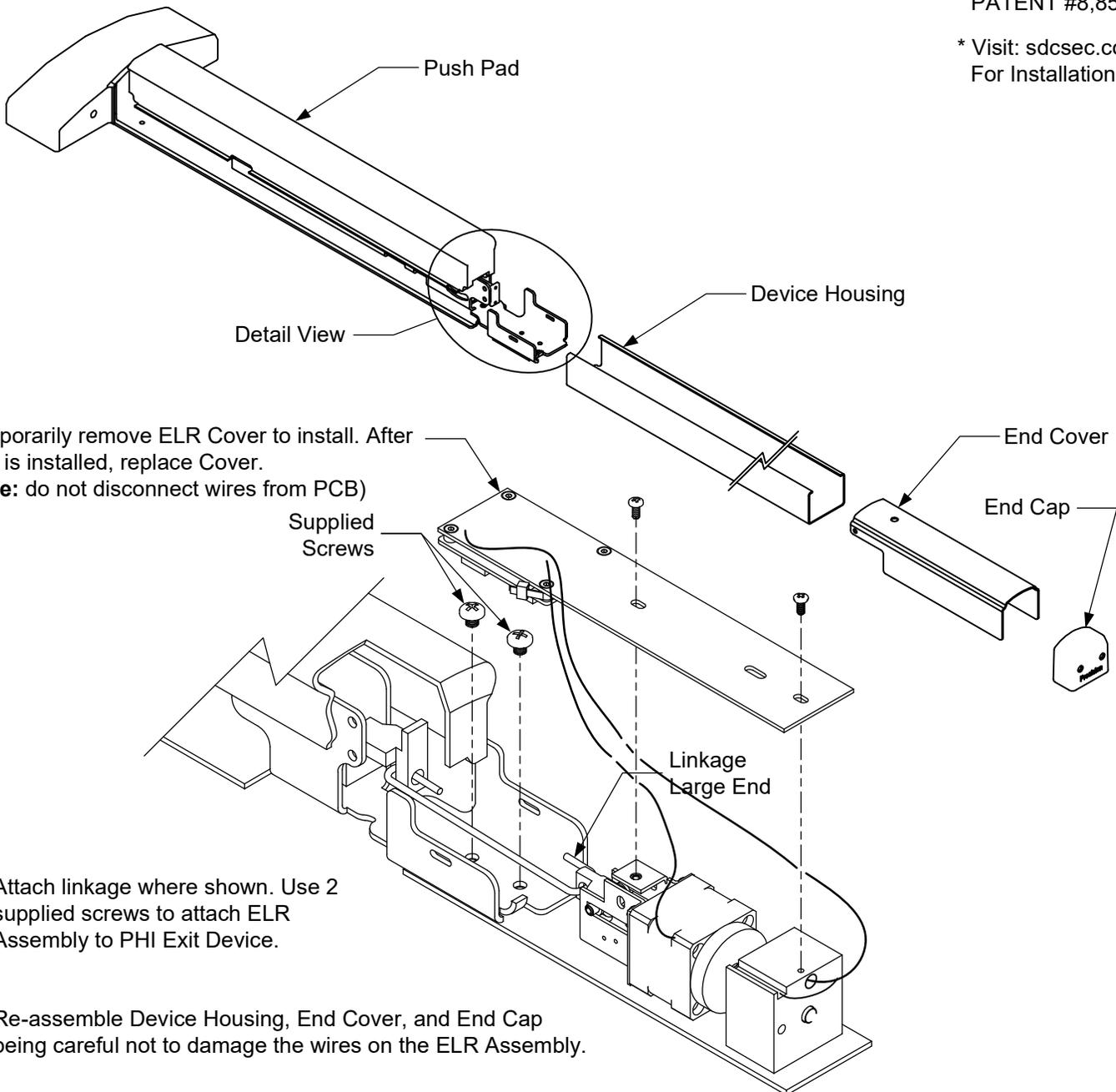
Temporarily remove ELR Cover to install. After ELR is installed, replace Cover.
