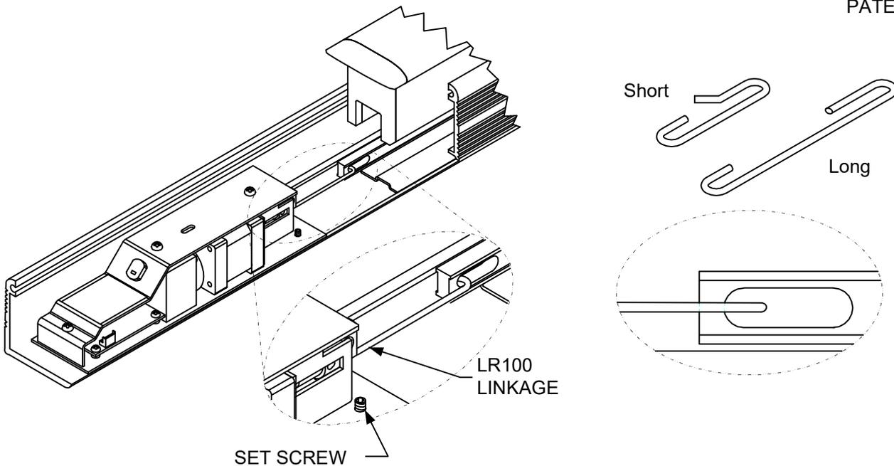
Back the assembly out until the linkage JUST makes contact with the latch retraction rod. Tighten set screws. Replace cover plate and end cap.
