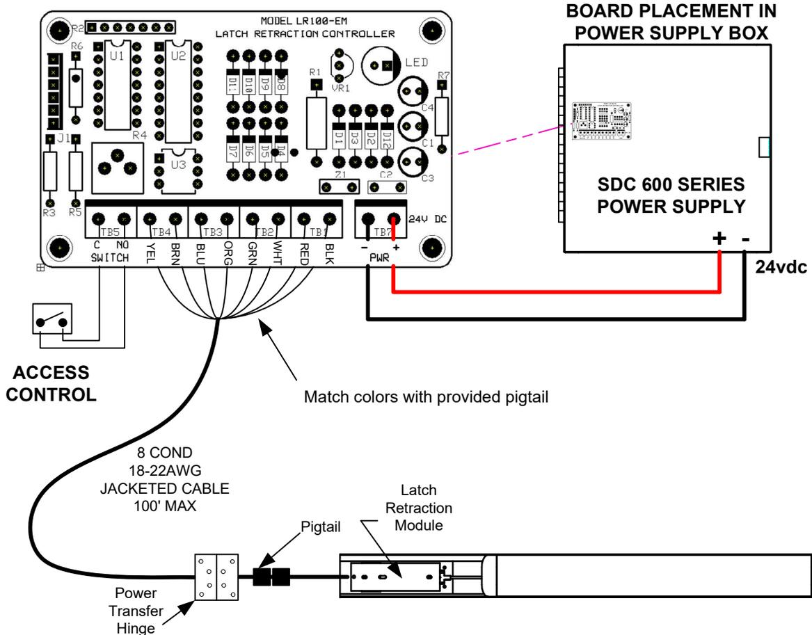
Wire colors from provided Pigtail must connect to the same colors marked on PCB. If the Jacketed Cable does not have the same colors as the Pigtail, use the following chart to mark the color connections from Pigtail to Jacketed Cable to PCB.
