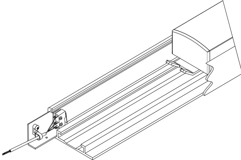
Tighten the set screw to lock the assembly in place. Release and depress touch pad several times to check that it is making proper contact with the switch.
