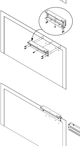
3. Install lock onto Frame Bracket assembly. Tighten integrated bolts to secure lock in position.
