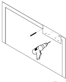
2. Assemble Frame Bracket & Lock Mounting Bracket. Install onto top of frame.
