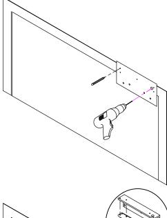
2. Assemble Frame Bracket & Lock Mounting Bracket. Install onto top of frame.
