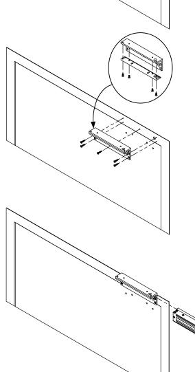
3. Install Lock onto Frame Bracket assembly. Tighten integrated bolts to secure Lock in position.
