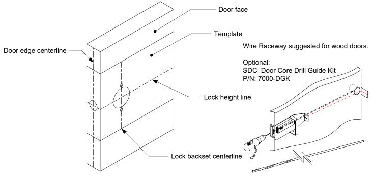
2. Drill out holes according to template. Standard commercial lock backset is 2-3/4" and residential backset is 2-3/8". Residential installations will require the 2-3/8" backset latch B2Q.
